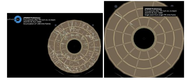
Event displays for 1000 TPC time frames (left) and a single reconstructed track passing through multiple TPC sectors (right). Data for both images comes from a single TPC data run (Run 10684, segment 0000) taken after first complete HV activation of the TPC in the IR.
