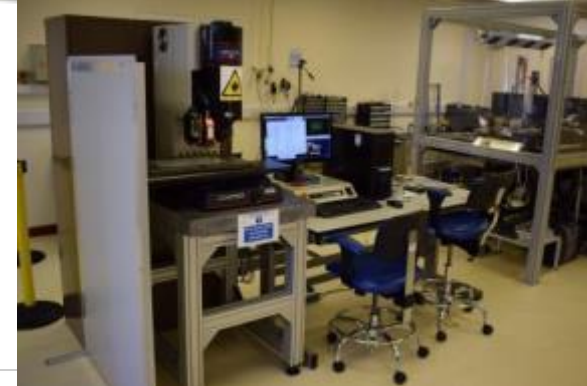
Pull/shear tester. XYZTec Condor 100
