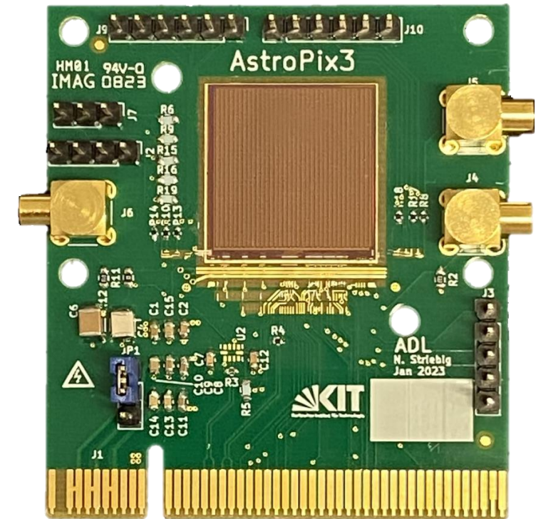
~2x2cm Astropix 3 Sensor placed on GECCO Carrier Board for Testing. Design by Nicolas Striebig @KIT, tests by Manoj Jadhav @Argonne and Amanda Steinhelb @NASA
