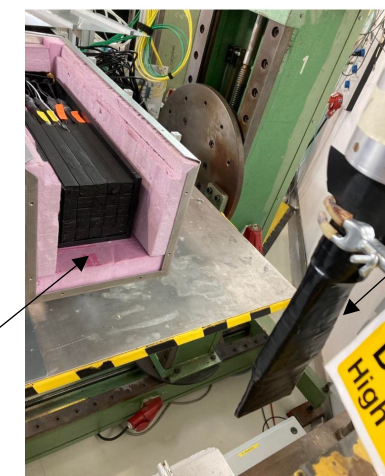
5x5 PbWO4 Crystal Array (2 cm 2 face) with 2-5GeV electron test beam
