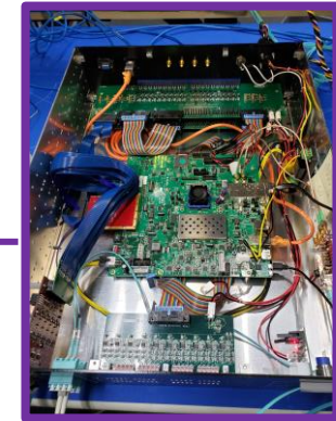
Global Timing Module (NSLS II/sPHENIX) Receiving from RHIC RF low jitter clock source
