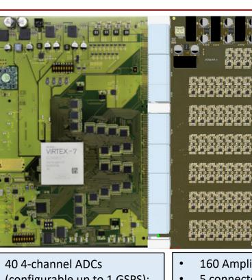
(configurable up to 1 GSPS); Single Virtex7 FPGA
