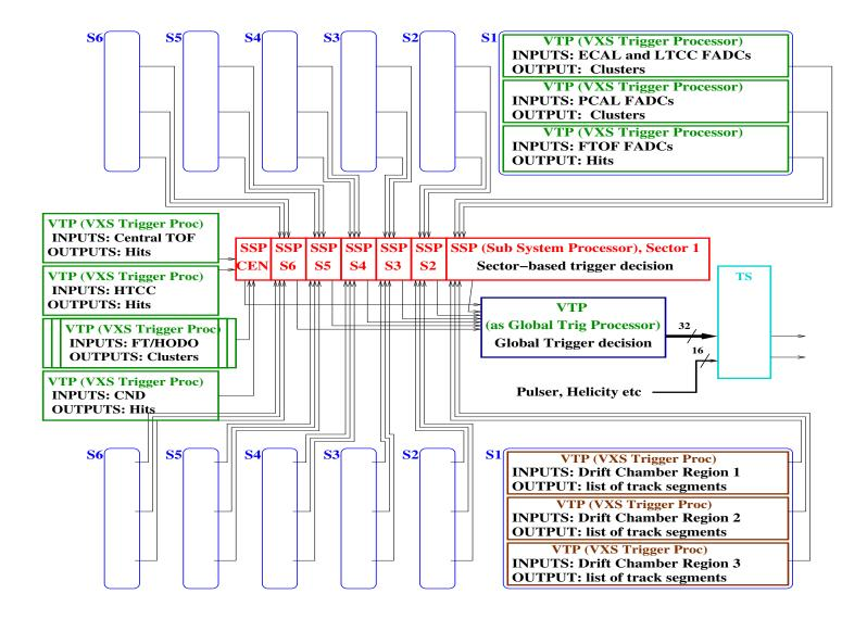
Trigger system core element: VTP boards (42 installed in CLAS12)
