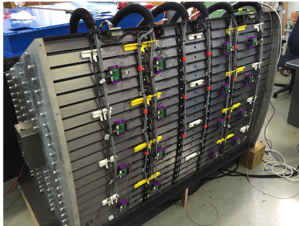
Figure 13: The fully assembled outer HCals sPHENIX test beam sector prototype. Each section has 20 steel absorber plates stacked together and 80 scintillating tiles are inserted between them. SiPMs read out from five tiles are ganged together like a tower in sPHENIX, but in the ePIC configuration each tile will be read out independently. This configuration is sufficient to contain a few GeV hadronic shower initiated in the center of the detector.
