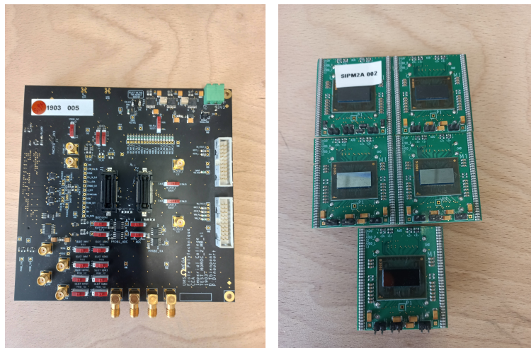
Figure 7: The carrier board (left) and the mezzanine board with the H2GCROCV3 (right)
