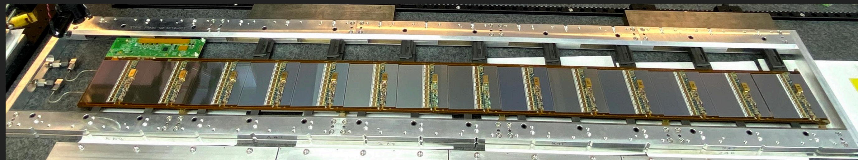
One side of the first 28 module stave prototype built with 50 \mu m accuracy
