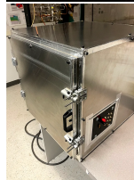
(a) Light-tight Faraday box with connector panel
