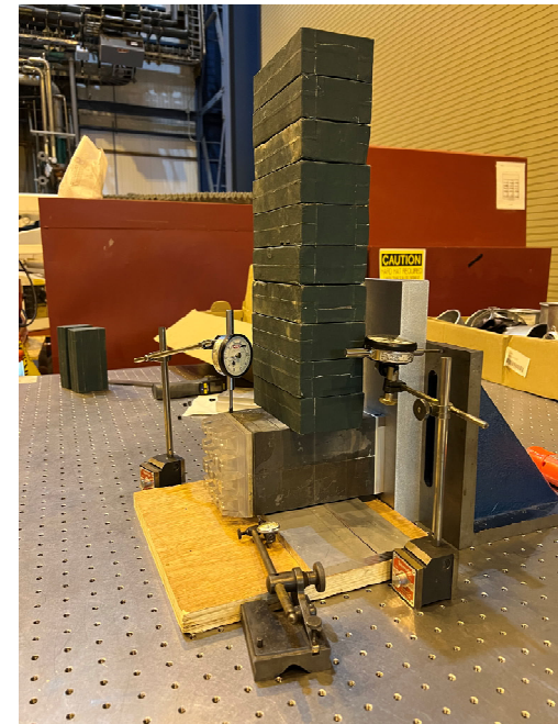
Last long term stability test at BNL. fECal installation block mounted on mockup fHCAL front plate, loaded x4 times nominal
