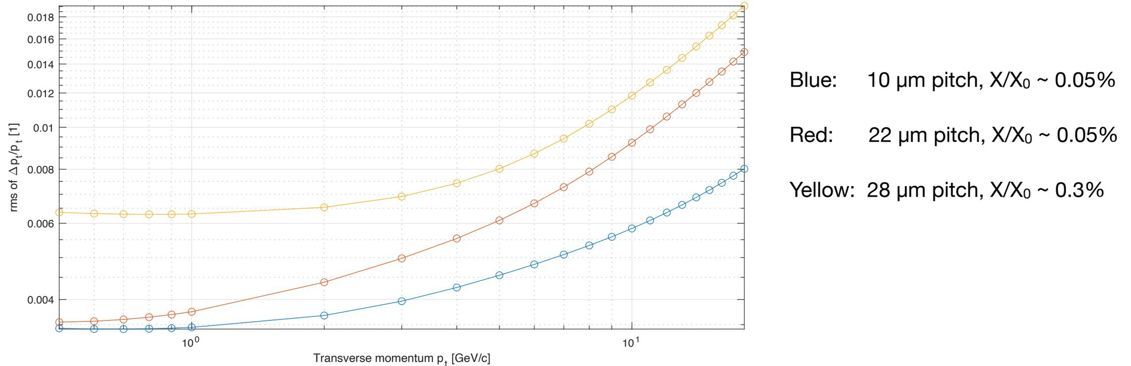
Point resolution and pixel pitch are proportional in these simulations; the usual factor of  $\sqrt{12}$ .
