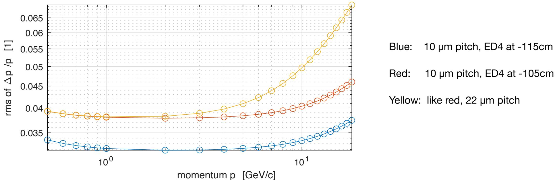
Note, disk ED0 is outside of the acceptance at this angle so that  $L \sim 60$  cm with ED4 at -105 cm, Effect of lever arm is  $\sim 19\%$  for 1 — 10 GeV/c and less than the ratio of  $L^2 \sim 35\%$ , Effect of pixel pitch is  $\sim 25\%$  at 10 GeV/c for a change in pitch from 10 to 22  $\mu\text{m}$ .
