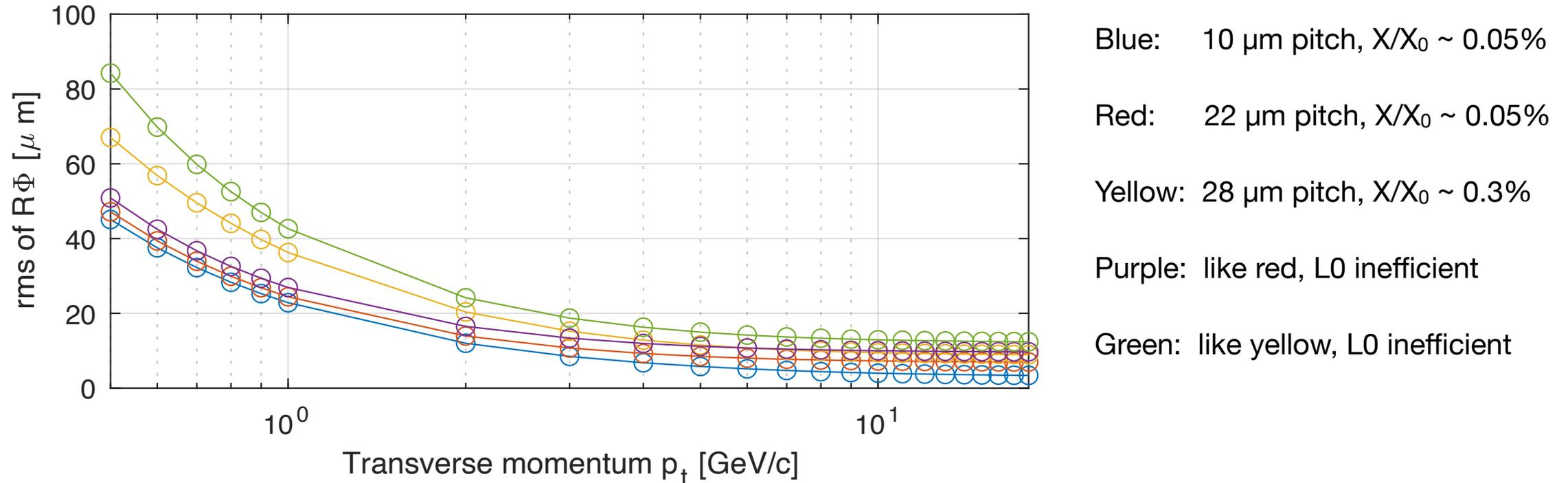
Point resolution and pixel pitch are proportional in these simulations; the usual factor of  $\sqrt{12}$ .
