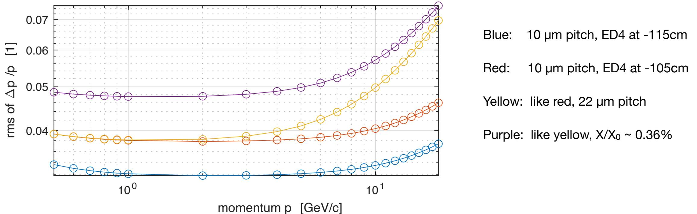
A  $\sim 25\%$  effect from a  $\sim 50\%$  increase in  $X/X_0$  at 1 GeV/c (indeed; expect  $\sqrt{\cdot}$ -scaling all else being equal),
