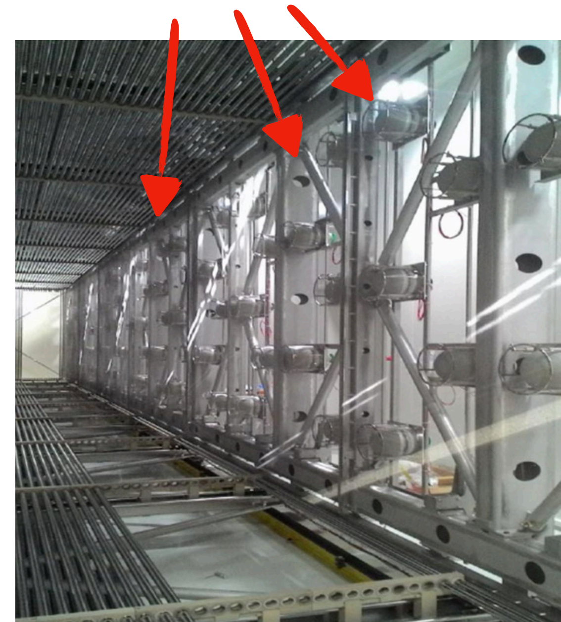
ICARUS Photo Multiplier Tubes (PMTs) on one of the walls
