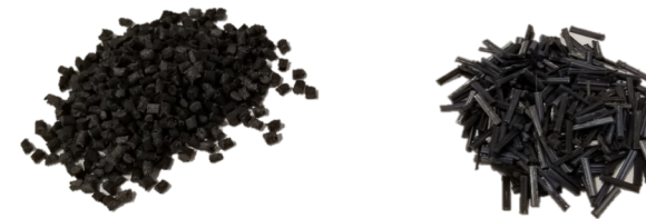
Feed Stock – CF short fiber filled Polyphenylene sulfide (PPS) OR Polyethersulfone (PESU)
