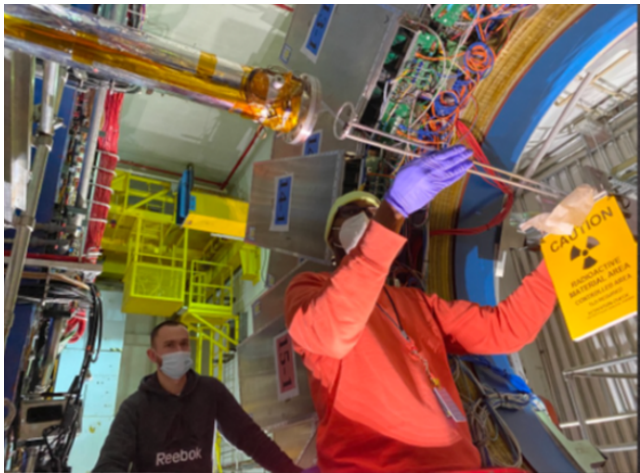
Figure 112: Left panel: Installation of the targets and holder on the East side of the STAR detector. Right Panel: A view down the beam pipe showing the three targets (C, Al, and Ni) installed at STAR.
