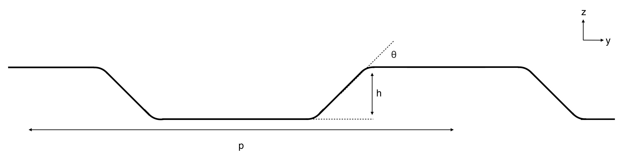
At least three relevant dimensions; pitch, height, and angle — others include length, thickness, ...
