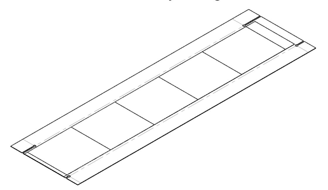
Note that the EIC LAS sensor here as five RSUs and peripheries on both sides. Its support extends slightly beyond the main periphery (likely needed for bonding) and the slots would allow for overlap along the length axis (provided the materials are all thin enough or the structure is not entirely flat).
