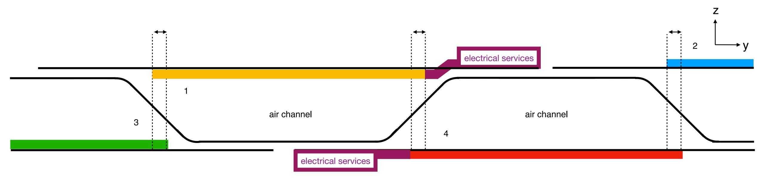
Having a sensor module part of the face-sheets — as shown here — would seem preferred, Arguments include that services can be guided to areas with mechanical support
