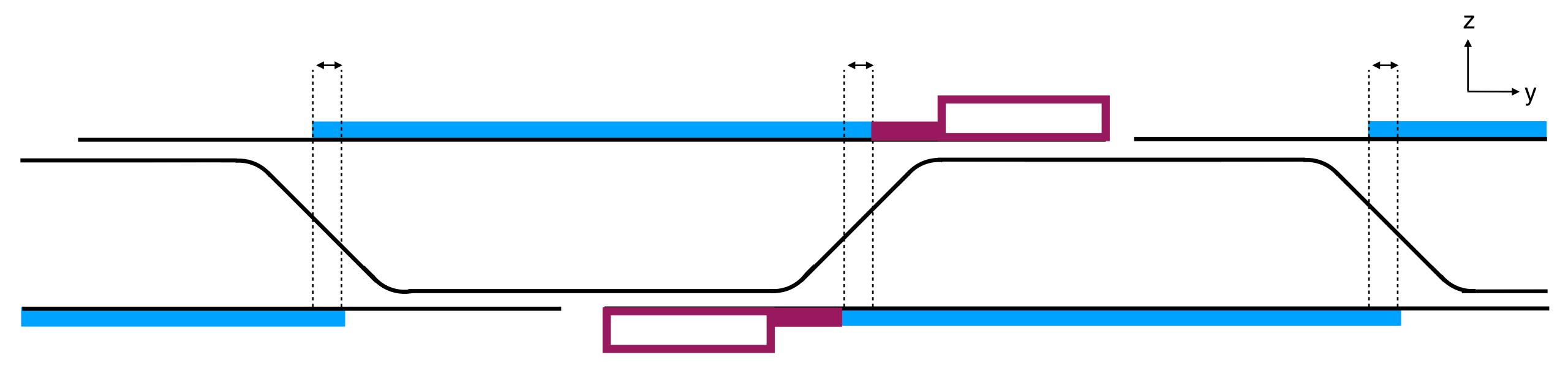
Having a sensor module part of the face-sheets — as shown here — would seem preferred, Arguments include that services can be *guided* to areas with mechanical support
