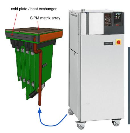
external chiller with fluid recirculation (ie. siliconic oil) the chiller here one is just a commercial example <u>https://www.huber-online.com</u> cooling and heating capacity could use heating capability for annealing? must be demonstrated to be feasible cooling capacity at -40 C is large (1.5 kW)
