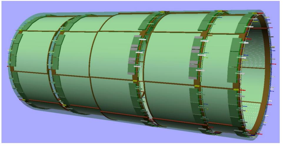
The green shade shows the **5.5 cm** radial keeping zone that would allow us to fit everything (FEB included) The design can be improved to fit in a slightly tighter region, but this is a "safe" assumption
