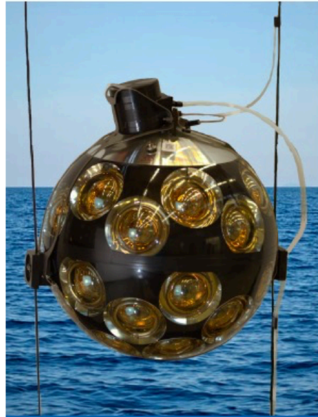
1 optical module = 31 photomultiplier tubes
