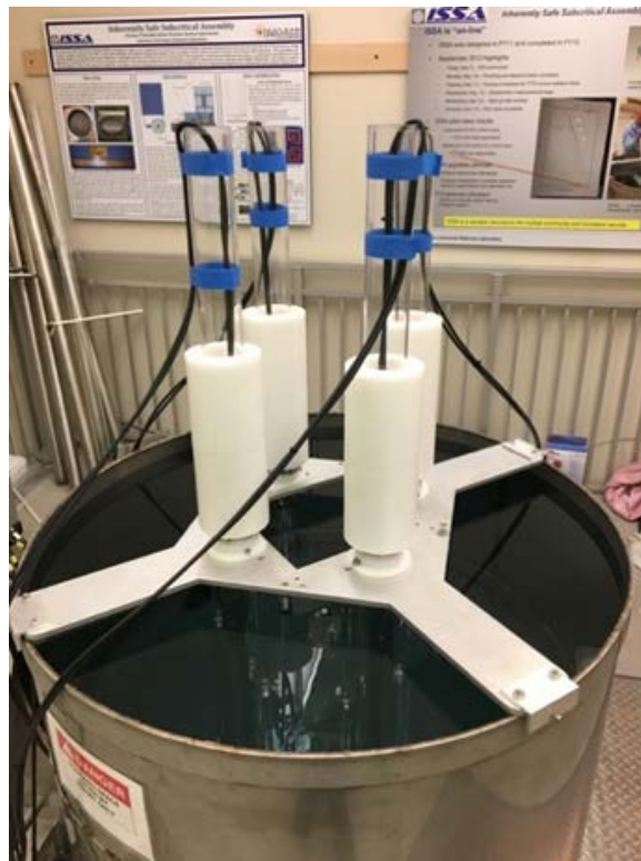
Figure 13: ISSA set up at B255 showing water tank and four He3 detectors
