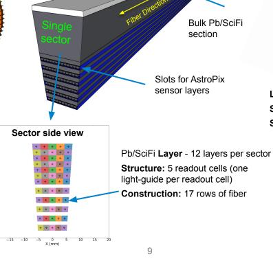
**Tray** - Structure holding the AstroPix staves for a single layer
