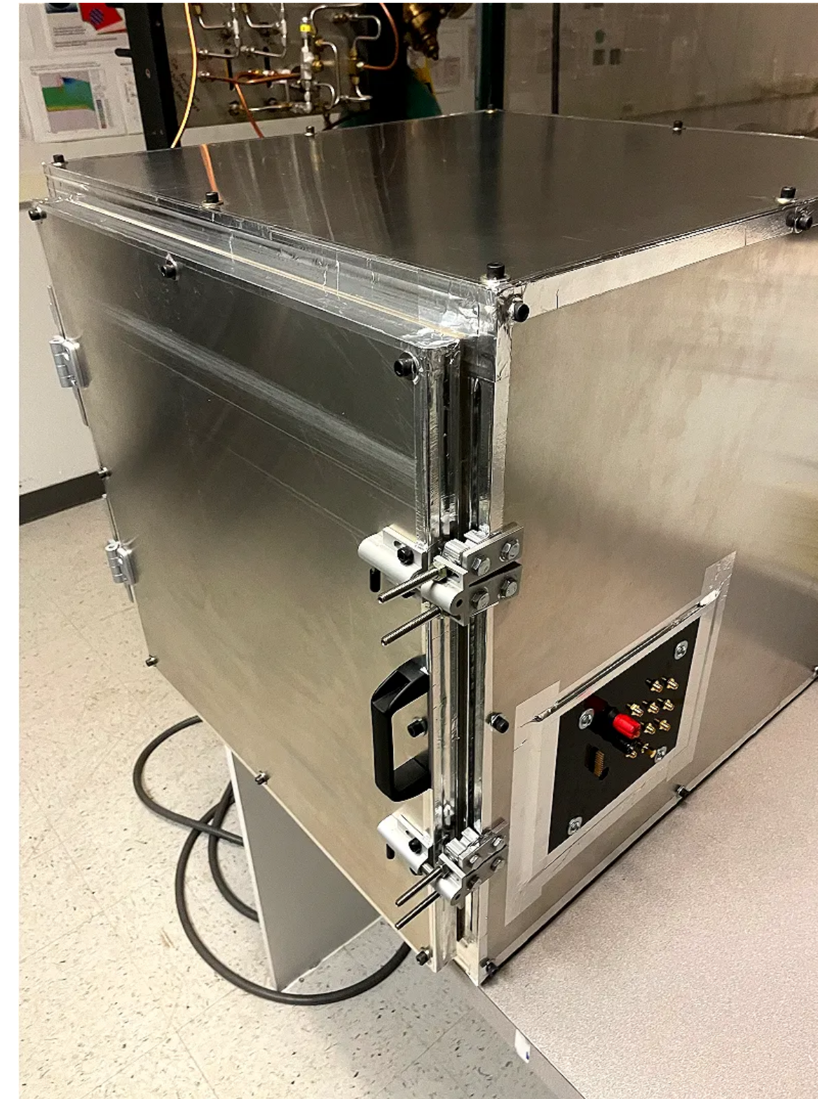
(a) Light-tight Faraday box with connector panel
