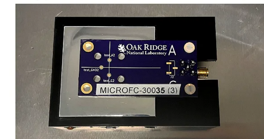
(e) Tile-SiPM holder with SiPM board
