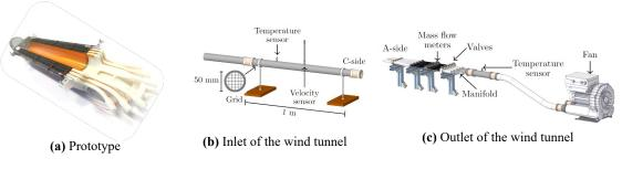
ALICE ITS3 cooling test setup
