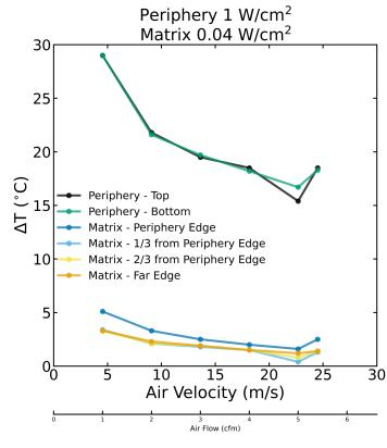
Uptick at highest velocity possibly due to thermocouple breakage
