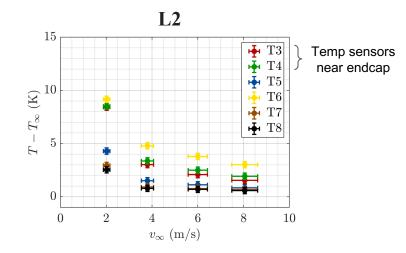
Measurements: endcap = 1 W/cm<sup>2</sup>, matrix = 50 mW/cm<sup>2</sup>
