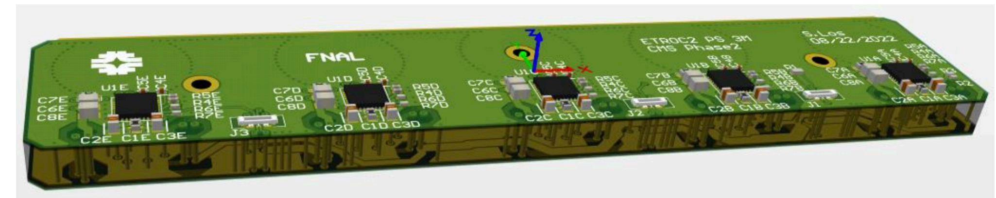
ETL front end power board
