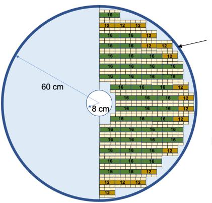
Cooling manifolds and LV/HV patch panels mounted on the rim of the DEEs to take advantage of space in the z direction and minimize impact to the active detector area
