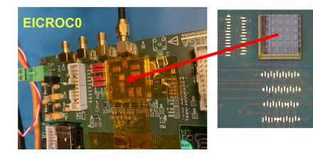
EICROC0 (4x4): first version ↓ EICROC1 (8x32?): intermediate size ↓ EICROC2 (32x32): full size ↓ EICROC3 (32x32): final (if needed)
