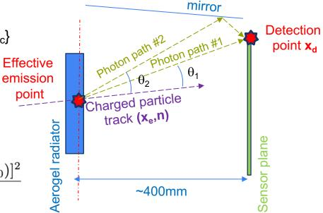
Path#1 and path#2 will not only have a different  $\theta_c$ , but a substantially different length (and therefore, a very different - compared to a ~50ps resolution flight time between the emission and detection points)
