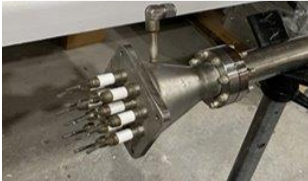
Feedthrough pressure and electrical tests completed
