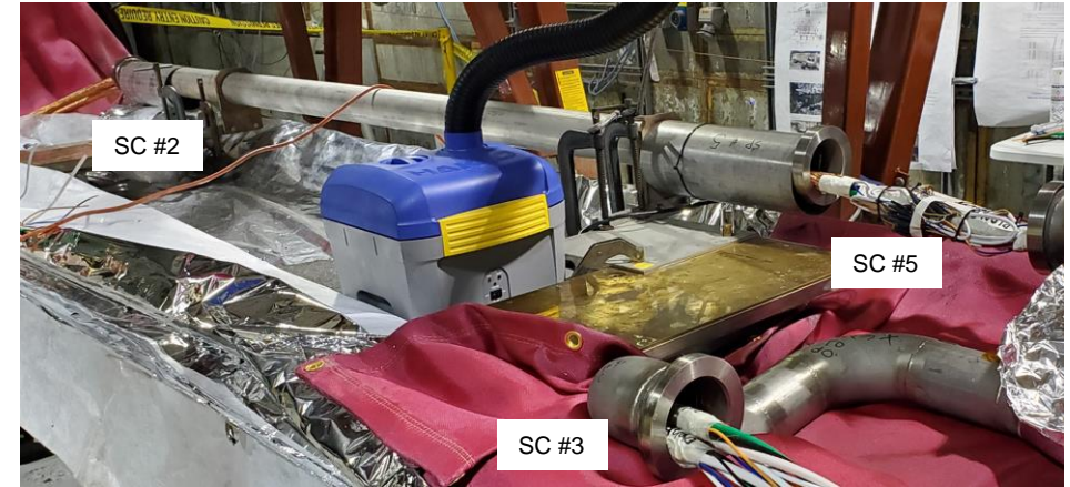
Electrical wiring: 3 “splice cans” (SC) completed, 2 prepared to accept DX magnet
