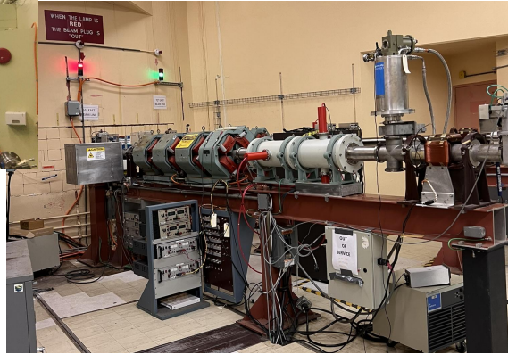
Beam pipe from Tandem Van-de graaff accelerator with proton beam.
