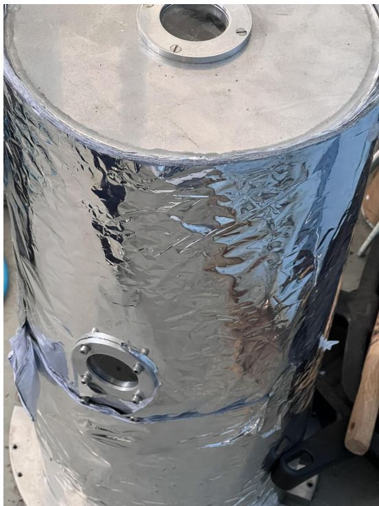
Layers of thin aluminium foils surrounding the vacuum cryostat.
