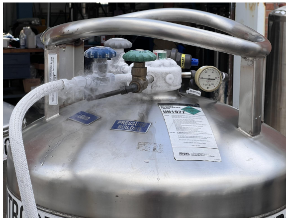
Liquid Nitrogen used for condensing Argon gas after purification.
