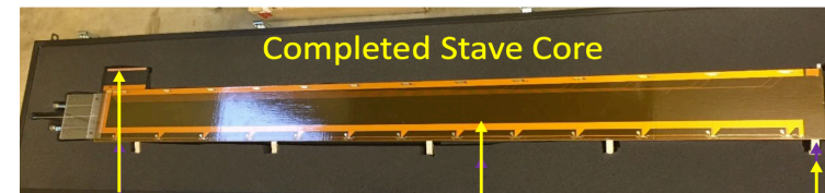
Copper ground strip in End-of-Stave region
