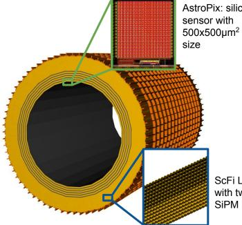
AstroPix: silicon 500x500µm<sup>2</sup> pixel
