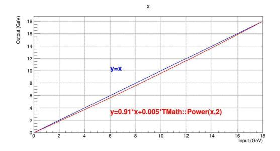
**Non-linearity of electronics**: preamp, ADC...
