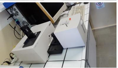
The CERN VSC (Vacuum Surface and Coating) Group has a chemical laboratory equipped with analysis instruments: Gas-chromatograph (60 m long column) with Mass Spectroscopy, IR and UV gas spectroscopy - UV transparency analyzer.
