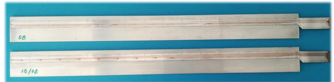
Multilayered flexible boards on carriers for FoCal 15-chip OB and IB/OB strings
