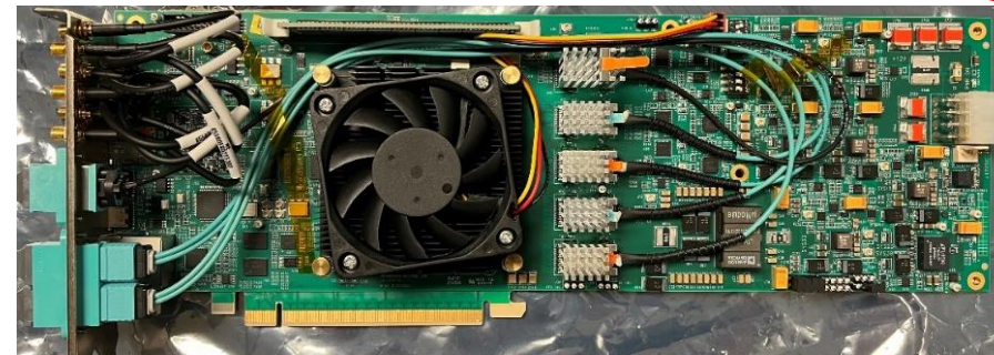
FLX 182 board Used for timing studies and DAM firm/software development
