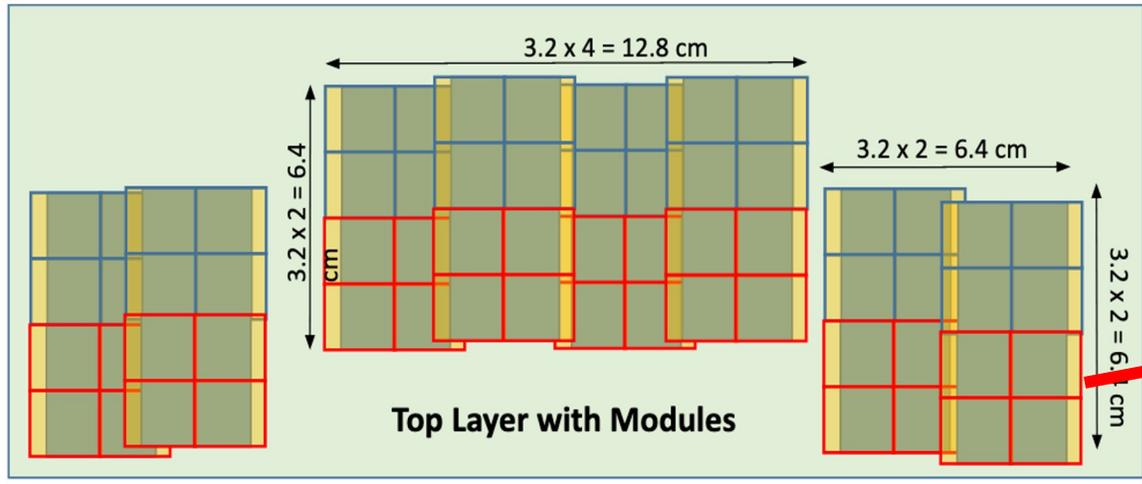
We are finalizing plans to likely move to a “one sensor, one ASIC” concept to simplify the sensor and module production.
