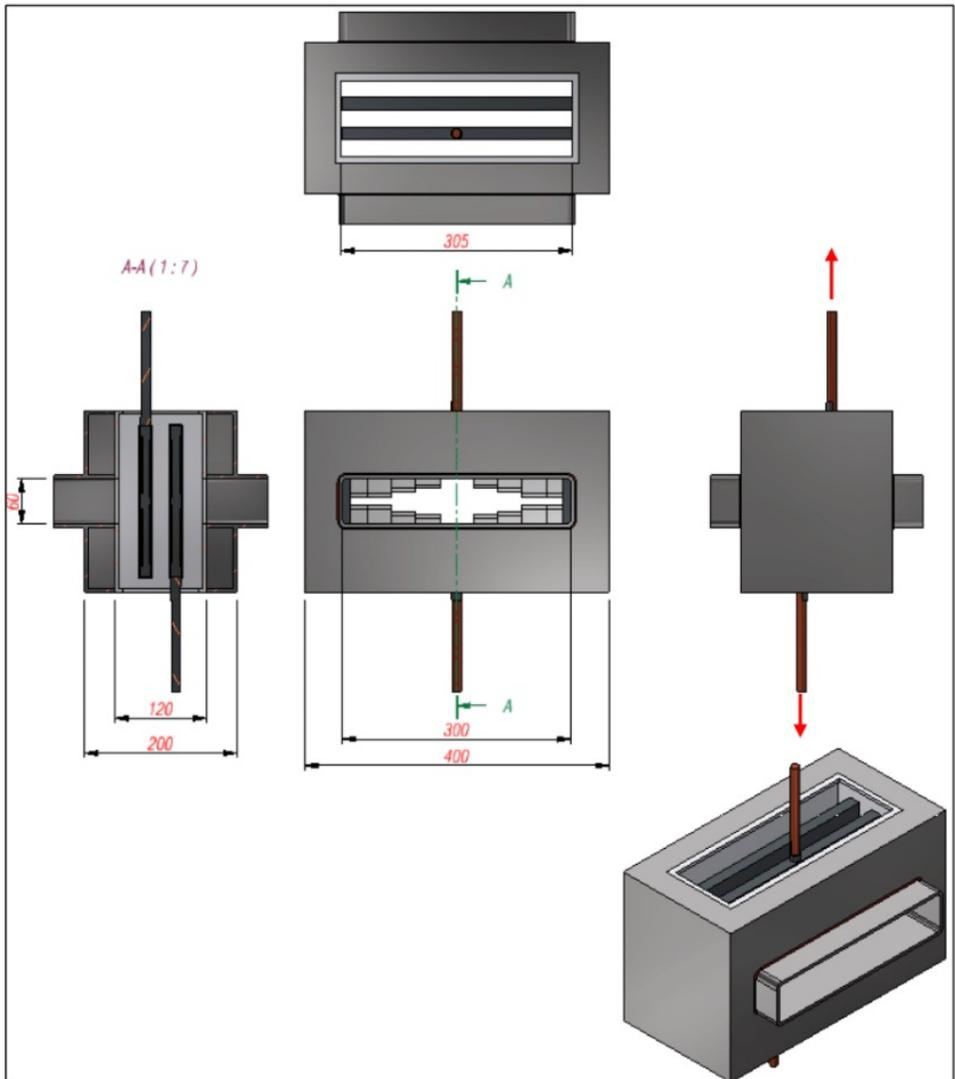
Scattering chamber design for RP sensor packages.
