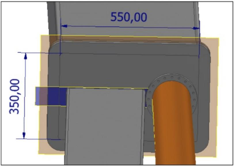
Transition region from larger beam pipe containing OMD to smaller pipe containing RP (left) and exit window for neutrals (right).
