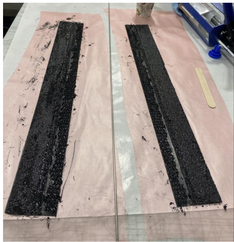
Apply Araldite 2011 mixed with 10% graphite by weight to each half of machined stave
