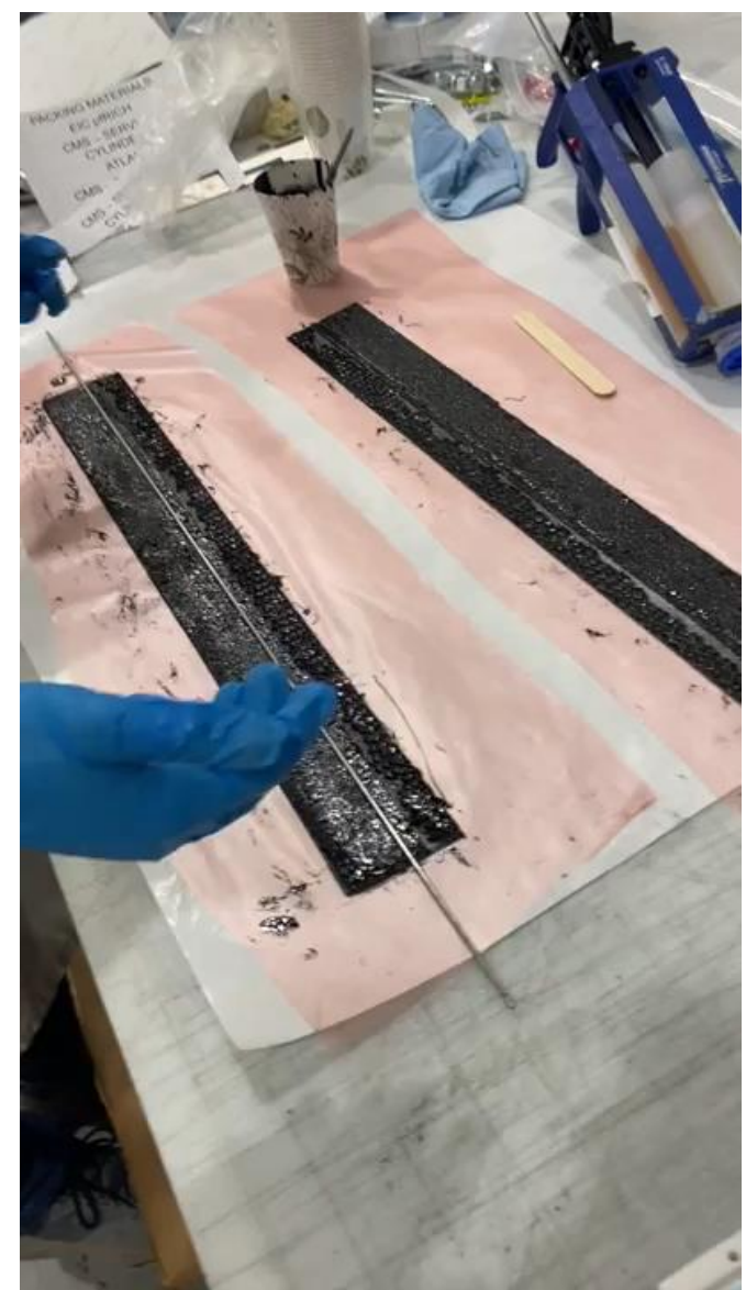
Join stave halves around coolant pipe
