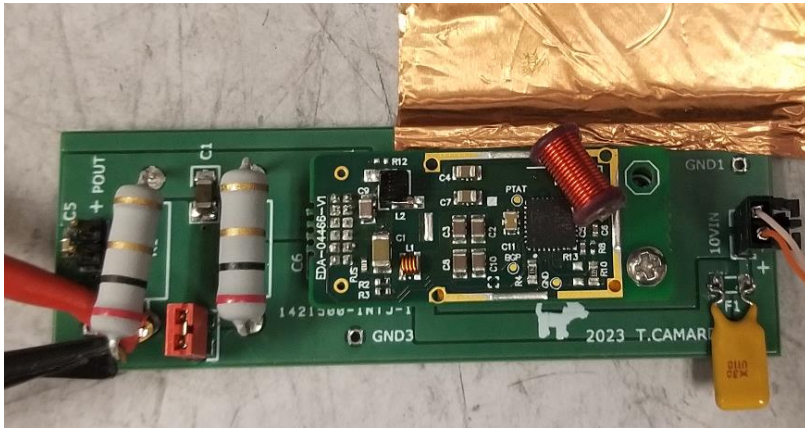
bPOL12V eval board mounted on test adapter carrier board
