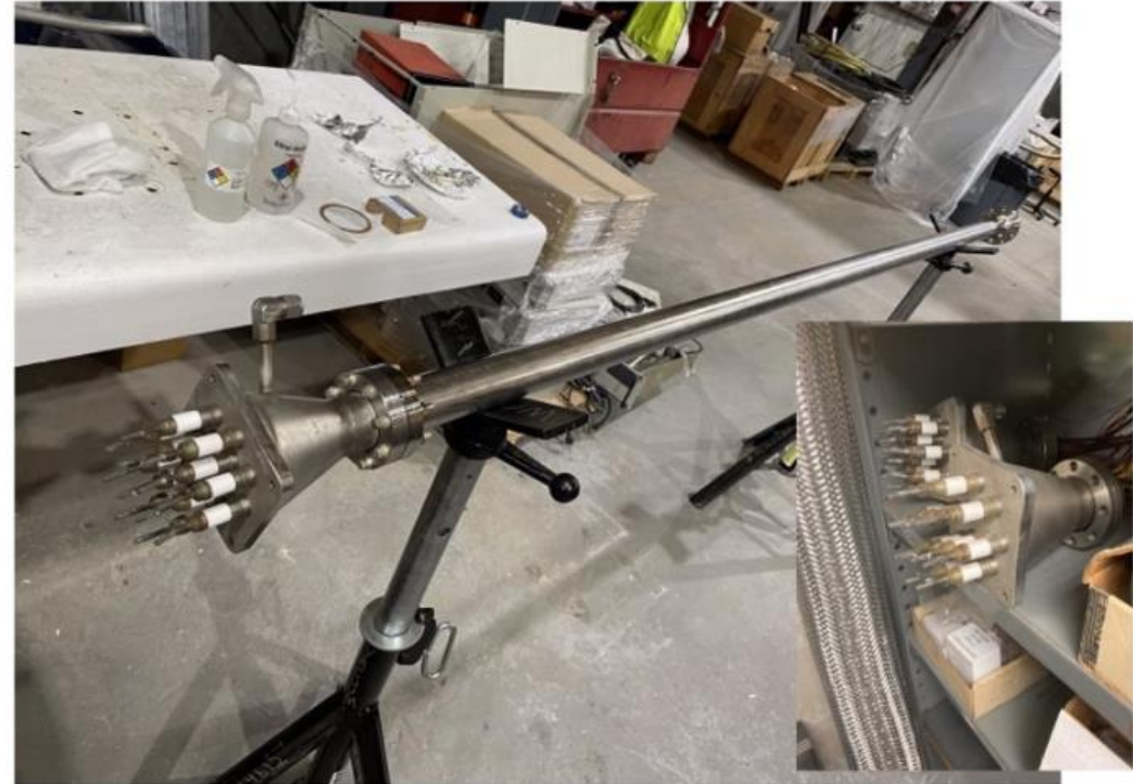
Vacuum test setup (using another, partially-built current lead)
