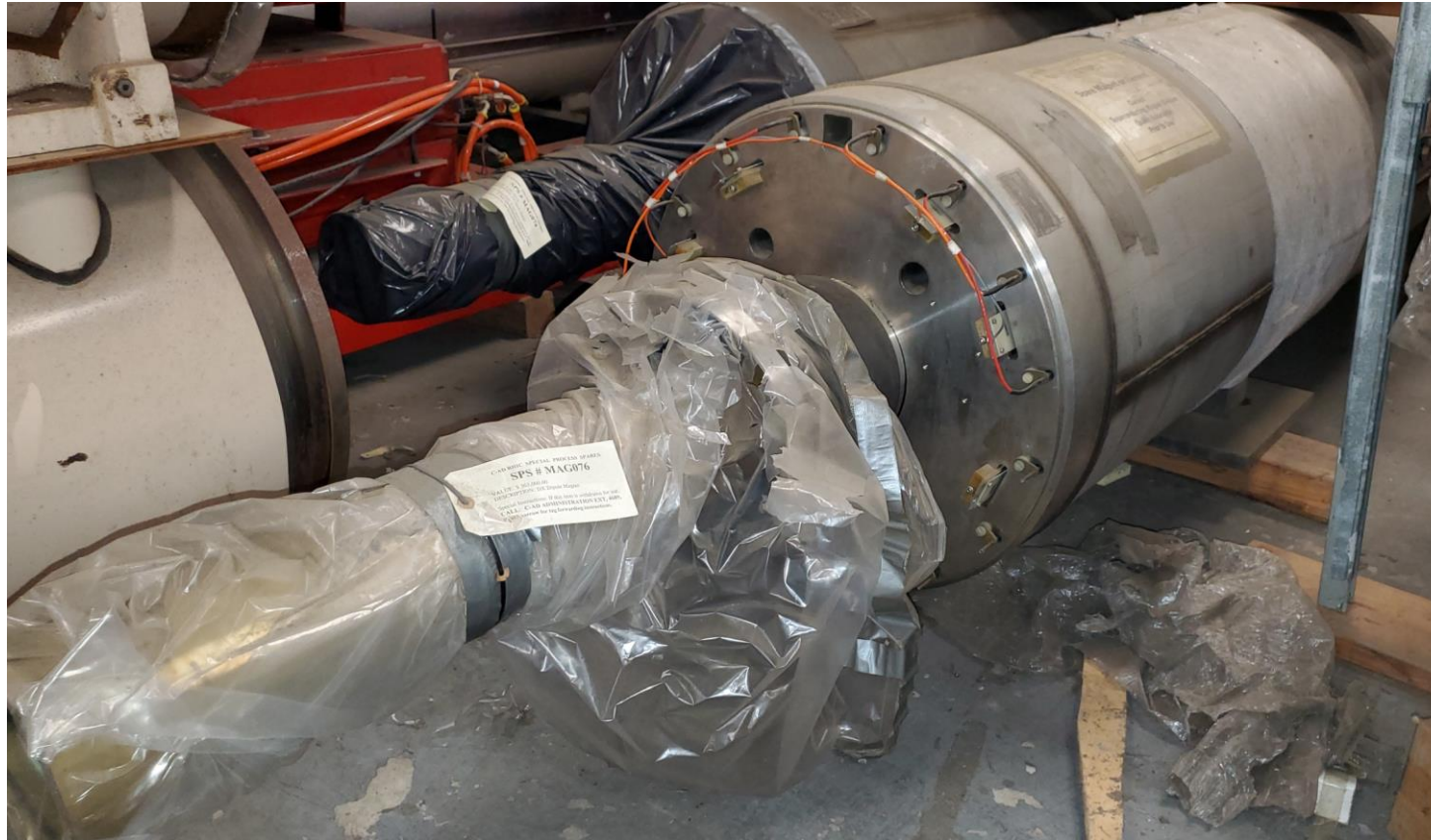
DX Cold Mass/Yoke assembly - without end volumes (from special process spares inventory)
