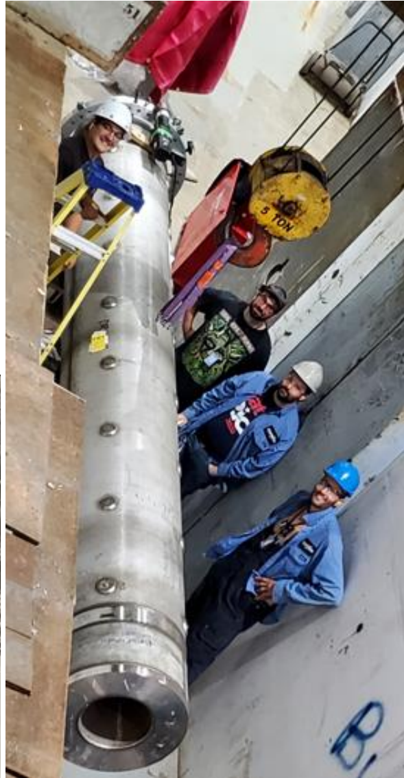
Pipe cutter (WACHS) used to grind off DX magnet end caps
