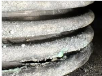
Feedthrough tube rupture
