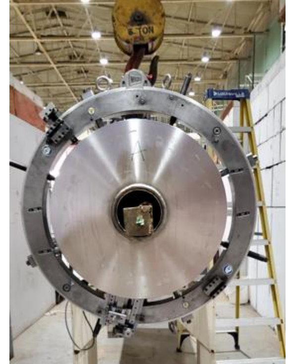
Pipe cutter (WACHS) used to grind off DX magnet end caps
