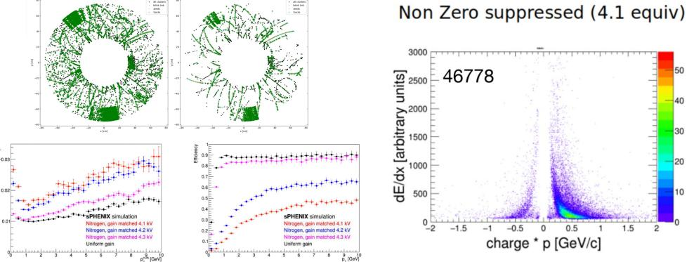
sPHENIX has worked with ESSHQ of C-AD and BNL SME in the USI process in order to use up to 5% isobutane to get to more efficient operating voltages for the TPC in sPHENIX.
