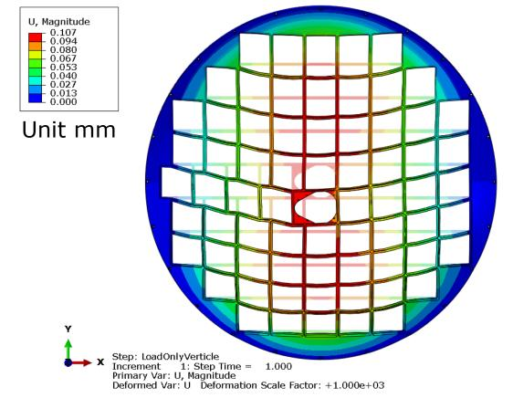
1000x the deformation shown to understand the trend in deformation
