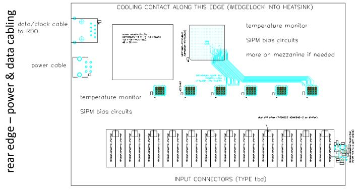
1 FPGA (Polarfire) 6 quad ADC's
