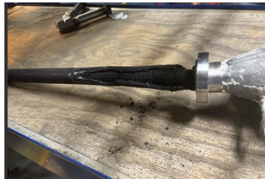
Damaged current lead
