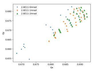
Although RHIC typically operates with protons at the beam-beam limit, operating with a crossing angle reduces the beam-beam footprint.
