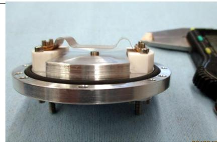
Prototype of the pulsed (isolated valve) for the gas injection to the extended EBIS.
