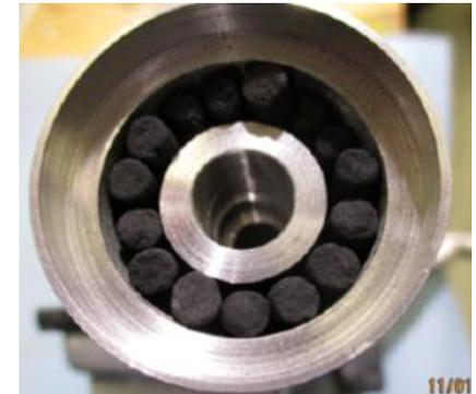
**Left:** "Open"  $^3\text{He}$  gas cell (30 mm in diameter) with the isolation (filling) valve attached
