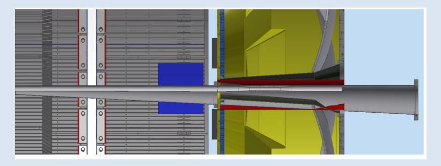
An asymmetric dRICH bore could be the solution, to be validated with simulations
