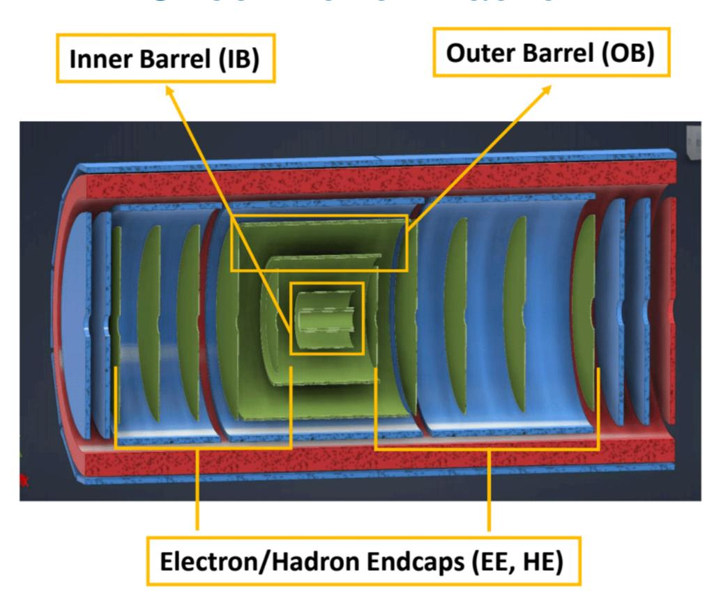
SVT Inner Barrel is based on ITS3 sensors,
