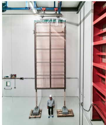
The DUNE anode wireplane assembly
