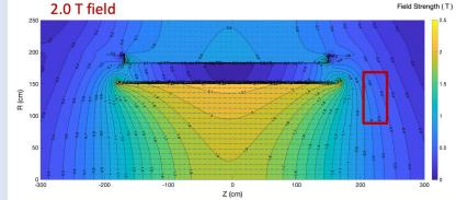
Strong (~ 0.7 T) magnetic field, not uniform Moderate radiation level (~  $10^{10} n_{eq}/cm^2$  after 1000 fb<sup>-1</sup>)
