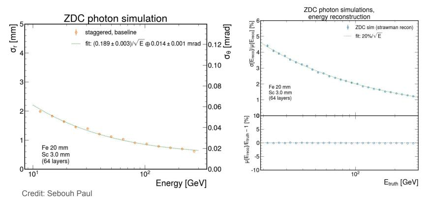
Fe/Sc SiPM is adequate for high-energy photons
